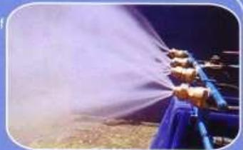
**Principle:** Water and Air are mixed internally to provide a fine fog. This fog gives a film of water coating on ultra fine dust particles, thus increasing their weight, and subsequently precipitating them. Each spray can be adjusted by air and water pressure changes to control spray / water density and throw of mist spray.
