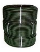
Our Drip Lateral is used in wide spaced crop for installing Emitters, Micro sprinkler, Foggers, Microsprayer for controlled irrigation. The high strength of its raw material LLDPE/LDPE assures durability under various UV degrading conditions. Available in sizes of 12mm & 16mm OD, having a pressure rating of 2.5 kg/cm2.
