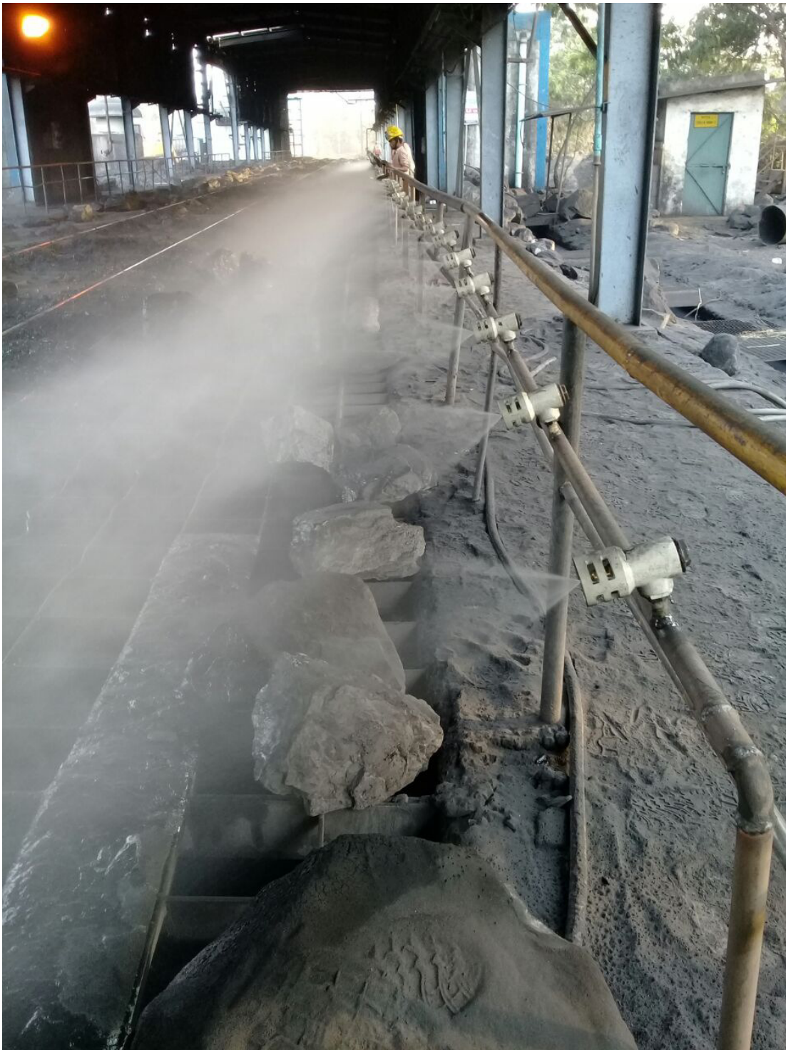
Eyeball Type misting Jet Nozzle with Housing in operation at Tracker Hopper
